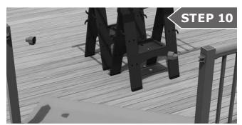
Position rail section with access to rail ends, then detach the bracket cups from the backer plates.
