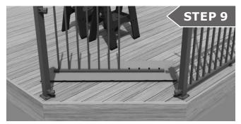
Assemble the rail section by first pressing the balusters onto the bottom rail nubs, then press the top rail nubs into the baluster tops. Use even force to fully seat all of the balusters.
