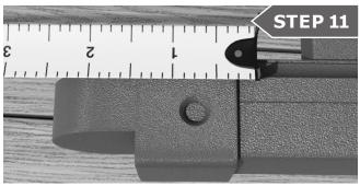
Place the bracket cups on the rails at both ends, leaving a 1/4" gap on each.
