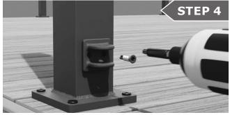
Place the angled bracket backer plate against the post horizontally at your mark and fasten to the post with two #14 Tek screws.
