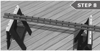
Place your rails on a fat surface, nubs side up, and mark your measurement with equal distances between the nubs, at both ends on both rails.
