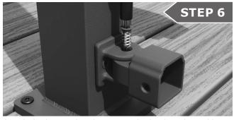
Attach the bottom bracket cup to the backer plate with a #14 Tek screw. Repeat the process for the top bracket.
