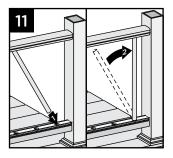
adaptor strip of bottom rail, maneuver baluster into upper rail aluminum baluster adaptor strip. Some force will be needed to press balusters into place and level them.
