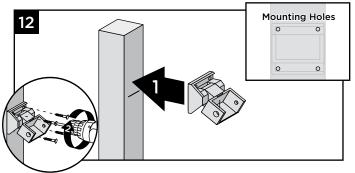
12. Remove upper stair rail from balusters and center upper stair swivel bracket on post **above** the marked line and attach using four self-tapping screws (provided).
