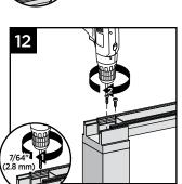
**NOTE:** Pre-drilling is recommended (7/64" [2.8 mm] drill bit) for attachment of railing to bracket.
