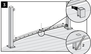
3. Temporarily set bottom rail into bottom brackets, and place Foot Block under bottom rail centered between bottom brackets. Mark to provide placement location of base. Remove bottom rail.
