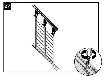
27. Install top rail to all vertical and end supports using ST Wedge Spacer and screws provided.
