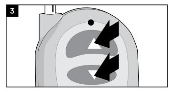
3. Press and hold both the up and down arrow on the dimmer remote simultaneously.
