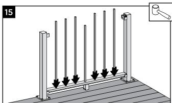
15. Place remaining balusters into holes in lower rail by snapping fully into place. In some cases, GENTLE tapping with a rubber mallet may facilitate fastening.
