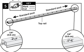
5. Cut each end of top rail 1/4" (0.6 cm) shorter than mark to allow for fit into top rail brackets.
