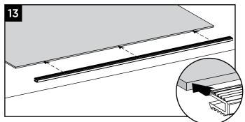
13. Lay glass on clean soft surface and install the bottom sill gasket onto the bottom edge of the glass panel.
