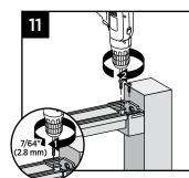
12. For crossover post configuration, fasten upper rail to crossover post by installing screws diagonally through upper rail into post using two selftapping screws each side (provided with bracket kit).
