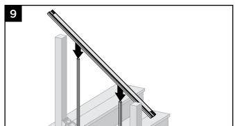
9. Position top stair rail onto balusters ensuring balusters are fully seated in top rail (position to side of post) and **ENSURE** that balusters are parallel with post.
