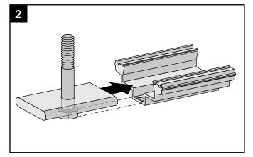
2. Align and insert the wedge plate with bolt into the v-wedge. Slide the wedge plate in until the ends are flush with the ends of the v-wedge.
