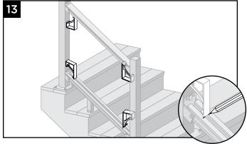
13. Using the long edge of the stair template, mark the location of the end verticals on the upper and lower rails.
