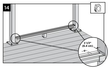
14. For full span installation, make a temporary mark on the bottom rail (example: use removable tape) 2-1/2" from each post. This will allow for glass to be centered between posts on bottom rail.
