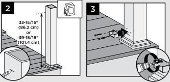
Measure up from decking surface 33-15/16" (86.2 cm) for 36" (92 cm) rail height or 39-15/16" (101.4 cm) for 42" (107 cm) rail height. Mark with light line.
