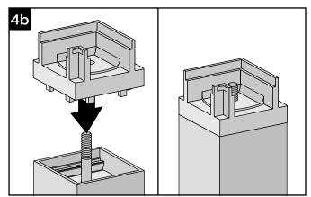
4b. Place the corner crossover bracket over the bolt onto the end of the post.
