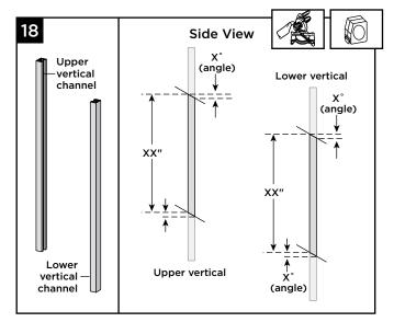
18. Ensure the verticals are oriented in the correct location, with the channels facing toward each other. Cut verticals to the dimension and at the angle provided above.
