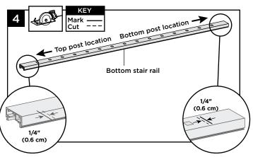
4. Cut each end of the bottom stair rail, rail insert, and bottom rail cover 1/4" (0.6 cm) shorter than the mark on each end to allow for fit into bottom stair rail brackets.
