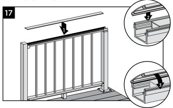
17. Attach "crowned" upper rail cover to upper rail by aligning cover on one side of rail. Then starting from one end of rail, snap cover onto opposing slot working down length of rail. In some cases, **GENTLE** tapping with a **rubber mallet** may facilitate fastening.
