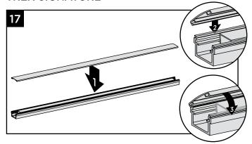
Attach "crowned" upper stair rail cover to upper stair rail by aligning cover on one side of rail. Then starting from one end of stair rail, snap cover onto opposing slot working down length of stair rail.
