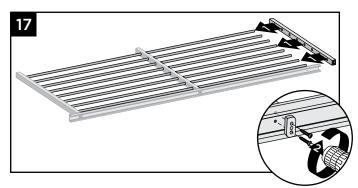
17. Slide end vertical onto rods and attach to bottom rail using HZ spacer and screws provided. HZ spacer should be oriented so the ribbed side of the spacer is not showing. TREX SIGNATURE RAILING
