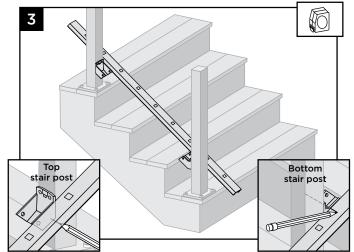
3 Position bottom stair rail along the nose of the stair treads. Ensure that before cutting, balusters holes are centered in between the posts and also allow for clearance for attachment to brackets. On top stair post location, mark **UNDERSIDE** of lower rail. On bottom stair post location mark **TOPSIDE** of lower rail at angled intersection of the bracket.
