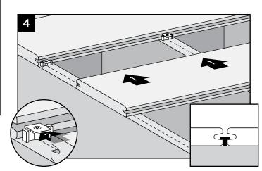
4. Install next board against installed hidden fasteners. Some slight force (using a rubber mallet) to seat next board against fasteners may be required.
