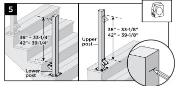
5. On Lower Post - From top of lower bracket, measure up and mark with light line (33-1/4" for 36" rail; 39-1/4" for 42" rail).
