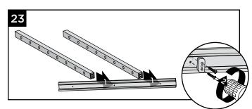
Install lowest end vertical and all intermediate verticals to bottom rail using ST Wedge Spacer and screws provided.
