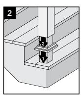
NOTE: Shims can be used to plumb post sleeves.
