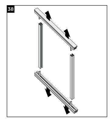
38.Disassemble stair rail panel.
