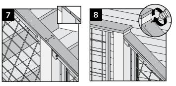
7. Use scarf cut for posts where two deck boards meet.
