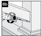
IMPORTANT NOTE: SET DRILL TO LOW SPEED AND LOW CLUTCH SETTING WHEN INSTALLING THESE SCREWS. DO NOT USE IMPACT DRIVER.
