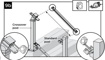
9b. When going from standard stair post to stair crossover post, measurement must be taken from inside of top horizontal stair swivel bracket to inside lip of stair crossover bracket. Crossover post will need to be modified to have swivel crossover bracket installed.
