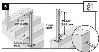
On Lower Post: From top of lower bracket, measure up and mark with light line (33-1/4" for 36" rail; 39-1/4" for 42" rail). On Upper Post: From top of lower (upper) bracket, measure up and mark with light line (33-1/8" for 36" rail; 39-1/8" for 42" rail).
