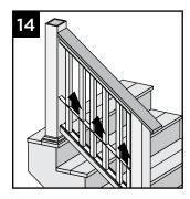
14. Slide baluster spacer up and snap into top rail.
