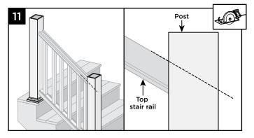
11. Cut post and post sleeves to proper angle so cut is flush with the top rail. Be careful to not cut top rail.
