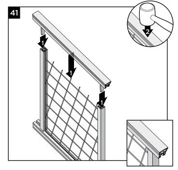
41.Align top rail with L-brackets, and press top rail down so that mesh panel is seated into gasket in channel and top rail is fully seated onto verticals. Use a rubber mallet to gently tap railing into place. TREX SIGNATURE RAILING
