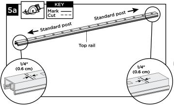
5a.Cut top rail to the measurement between the top swivel brackets. For standard post-to-standard post configurations this would be same dimensions as that of the bottom rail.
