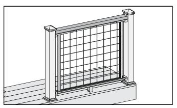
**Important: Only** use with Pressure-treated post, Trex Post Mounts or Trex Joist Mount Post WITH Trex post sleeves. Trex Signature Posts and Joist Mount Posts cannot be used with Mesh Traditional. 20. Use scarf cut for posts where two deck boards meet.
