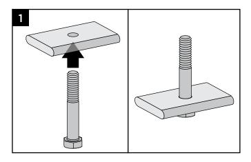
1. Insert the bolt through the hole in wedge plate.
