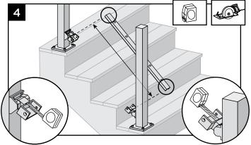
4. Cut each end of the bottom rail, rail insert, and bottom rail cover at the mark on each end to allow for fit into bottom stair rail brackets.
