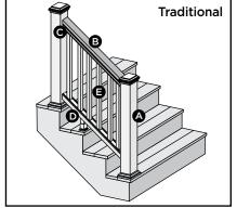
Cutting post sleeves is **NOT** required. Ensure both top and bottom post/post sleeves are tall enough to accommodate top rail and 2 x 4.
