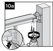
Attach attach top rail to bracket using two selftapping screws each side (provided). Screw from the bottom up into the top rail.
