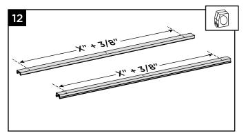
Measure the distance between the end (outer) holes (X") on top or bottom rail and add 3/8" to this measurement.
