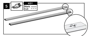
5. Cut both bottom and top rail to length as determined in previous step.
