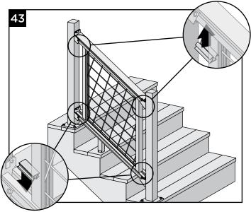
43.Cut snap-in channel filler to correct length and install into channels of bottom and top stair rails. Use of a rubber mallet may assist with this step.
