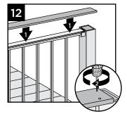
13. Secure boards to top rail using Trex Signature Cocktail Bracket (sold separately). Ensure that there is a bracket at each end of the railing section, then space brackets approximately every 24" and attach with 4 screws provided.
