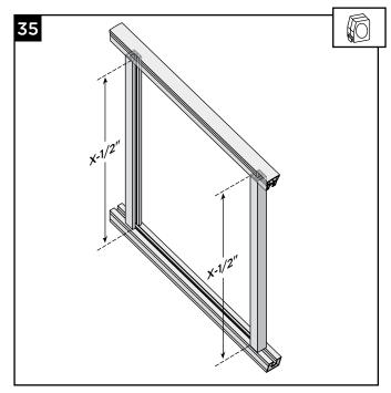
35.Measure distance within the channel of vertical and subtract 1/2".
