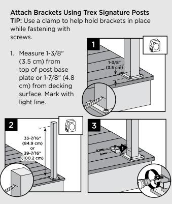
Measure up from post base plate 33-7/16" (84.9 cm) for 36" (92 cm) rail height or 39-7/16" (100.2 cm) for 42" (107 cm) rail height. Mark with light line.
