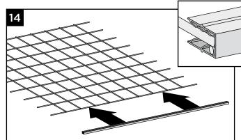
14. Install bottom PVC gasket onto bottom of mesh panel. Make sure gasket is fully seated onto mesh.
