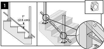
Lay bottom stair rail on steps beside posts. Position bottom rail at least 1" (2.5 cm) above nose of stair tread.
