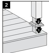
**NOTE:** Shims can be used to plumb post sleeves.
