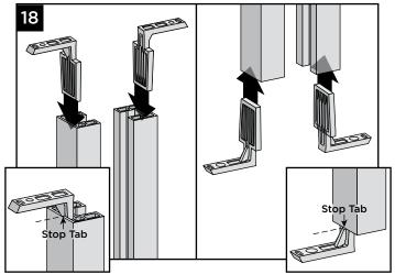
Install L-brackets into both top and bottom slots of vertical supports as shown. L-brackets will require light tapping until stop lip of bracket is resting on vertical support.
