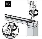
diagonally through upper rail into post using two self-tapping screws each side (*provided*).
