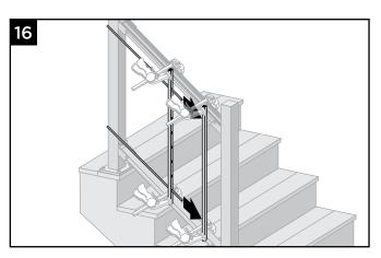
16. Slide a rod into top and bottom of all verticals. Ensure that distance of top rod to top rail and bottom rod to bottom rail are equal.
