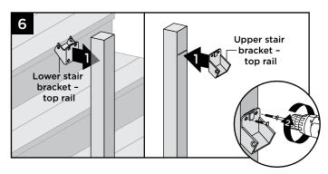
6. Center upper stair brackets on posts **below** the marked lines and attach using two #10 x 5/8" self-tapping screws (*provided*).
