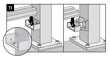
11. Place adhesive strips (provided) into bottom rail brackets, and then place bottom rail into brackets.
