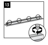
14. Place inverted universal rail with deck board attached over RSBs and glass panel. Attach universal rail to RSB's with three self-drilling screws provided (use three outer holes; do not use hole in RSB that is closest to post).
