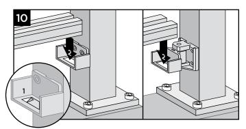
Place adhesive strips (provided) into bottom rail brackets, and then place bottom rail into brackets. Using a 3/8" drill bit, drill weep holes through center of bottom rail channel at 4 evenly spanned locations to allow for water drainage.
