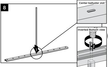
8. Attach shorter, center baluster in center slot in bottom rail using two #8 x 1-1/4" (3.2 cm) screws (provided).
