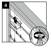
**NOTE:** Pre-drilling before attachment is recommended.
