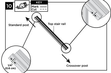
10. Top stair rail must be cut differently on each side of the rail. Railing side that attaches to standard post should be cut 1/4" (0.6 cm) shorter than the mark to allow for fit into top rail bracket. Railing side that attaches to the crossover post should be cut directly on the mark to allow for fit into the crossover post bracket.
