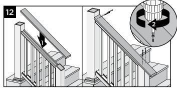
12. Place deck board on top rail and attach board to posts using two Trex recommended composite decking screws (use two screws per each post).
