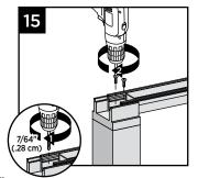
rail into post using two self-tapping screws each side (provided).
