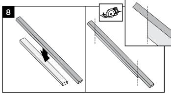
8. Using the cut top rail as template, cut 2 x 4 at same angle and length of the top rail.
