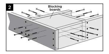
2. Install two 2" x 8" (51 mm x 203 mm) boards as blocking under post location. Securely attach blocking using a total of 24 3" (76 mm) pressuretreated compatible screws *(not provided)*.
