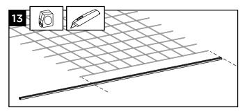
13. Using razor knife, cut bottom PVC gasket the same length as mesh.
