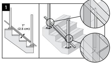
Place a 1" deck board on the nose of the stair tread, then lay the bottom stair rail on top of the deck board. Use the lower and upper stair post to set the size of the lower stair rail. On UPPER STAIR POST, mark from underside of bottom rail. ON LOWER STAIR POST, mark from top side of bottom rail.
