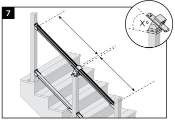
7. Determine location/height of the stair crossover swivel bracket by aligning the angle of this with the fixed brackets already installed. Note that the crossover post may need to be cut to ensure the top stair rail is parallel to the bottom stair rail.
