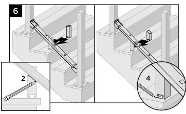
6. Temporarily set bottom rail in bottom brackets, and place Foot Block towards the nose of the stair tread along the side of the bottom rail. Mark location of angle on Foot Block and cut on mark. Then place Foot Block under the center of the bottom rail. Mark placement location of the base. Remove lower rail.
