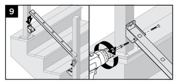
9. Set bottom stair rail into bottom stair rail brackets. Attach bottom stair rail to bottom stair bracket using two self-tapping screws (*provided*) on each side of bracket.
