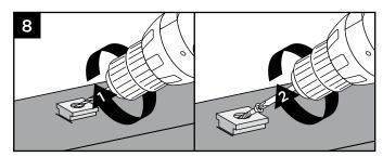
8. Remove bottom rail from lower brackets. Place base (smaller side facing down) on decking surface. Predrill using a 3/16" bit. Attach base of Foot Block using one screw at an angle through base and into decking.
