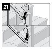
22.Attach provided post skirt to bottom of posts when using Trex Signature posts.
