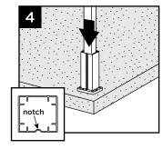
Attach bottom guide block using one 10 x 1" (25 mm) self-tapping screw (provided) in notch to lock guide block onto post.
