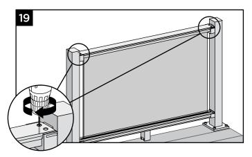
19. Using 9/64" bit provided, center into above holes and **PREDRILL** into top rail bracket at a depth of approximately 1-1/4". Use care to not drill through underside of top bracket.
