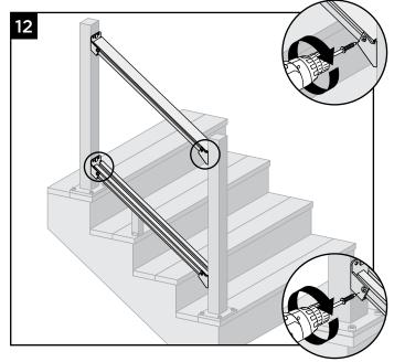
12. TEMPORARILY ATTACH BOTH BOTTOM AND TOP RAIL (IN ONE LOCATION ONLY TO ENSURE RAILS DO NOT MOVE) USING ONE #10 X 1" SELF-TAPPING SCREW (PROVIDED) ON SIDE OF BRACKET. YOU MUST PREDRILL THIS LOCATION FIRST USING 9/64" BIT THAT WAS *PROVIDED* IN HORIZONTAL MOUNTING KITS.
