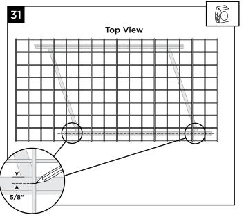
31.At inside of bottom rail, measure **DOWN** 5/8" and mark mesh at this location. Do this at opposite end of mesh panel/bottom rail. Using straight edge, mark **MESH ONLY** at all intersection points.
