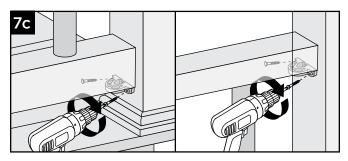
7c.Install both bottom and top brackets on each side to post using two #8-10 x 2" wood screws (*provided*).
