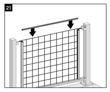
21. Install cut gasket onto top of mesh panel. Make sure gasket is fully seated onto mesh.
