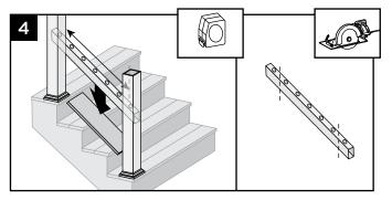
4. Set railing on top of deck board, making sure baluster holes are vertically aligned and mark line at each intersection. When measuring, cut equal lengths from each side of railing allowing a minimum of 2" (51 mm) on each end from the last baluster hole to the end of the rail. This will ensure proper baluster and bracket placement and equal spacing of balusters per each railing section.
