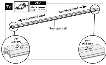
7a. Cut each end of top stair rail along with rail insert 1/4" (0.6 cm) shorter than mark to allow for fit into top stair rail bracket.
