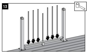
13. Place remaining balusters into holes in lower rail by snapping fully into place. In some cases, GENTLE tapping with a **rubber mallet** may facilitate fastening.
