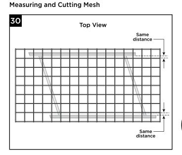
30.Lay mesh panel on top of stair rail assembly and measure so there is equal spacing between mesh panels at both top and bottom rails. Use clamp to hold mesh in place securely once dimensions are set.
