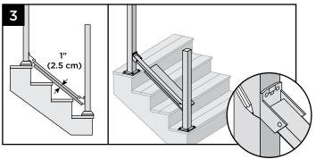
3. With deck board still on nose of stair tread, place brackets on end of bottom stair rail (DO NOT attach brackets to rail) and mark posts for bracket locations.
