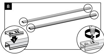
8. Place HZ template at end of top and bottom rails. Pre-drill pilot holes (using a 7/64" bit or small punch) at locations.
