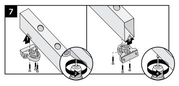
7. On the BOTTOM RAIL, attach the assembled bottom stair brackets to the OPPOSITE SIDE of the baluster holes. Attach both brackets using three #8-18x1" selfdrilling screws (provided).
