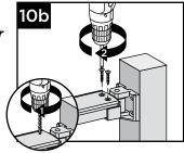
this on opposite side of top rail. Using a 7/64" (0.28 cm) drill bit, pre-drill at marked location for attachment of railing to bracket. Attach top rail to bracket using two self-tapping screws on each side (provided).
