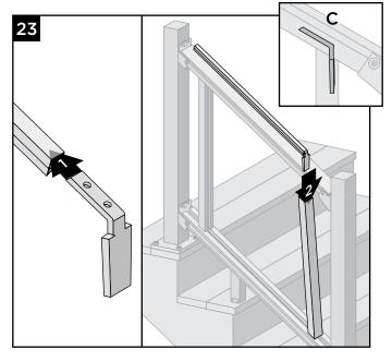
23.**At BOTTOM POST LOCATION**, slide L-bracket into end of gasket. Slide L-bracket (with gasket attached) into top of vertical.
