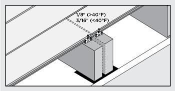
**NOTE:** Optional - Gap joist framing 1/8'' - 3/16'' to allow for water drainage.
