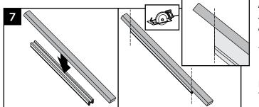
7. Using the cut top rail as template, cut 2x4 at same angle and length of the top rail.
