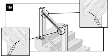
19. Mark both posts on inside channel of the top stair rail. Remove top stair rail.
