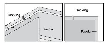
Install fascia UNDER decking edges/ends. This will optimize the aesthetics of the installation.
