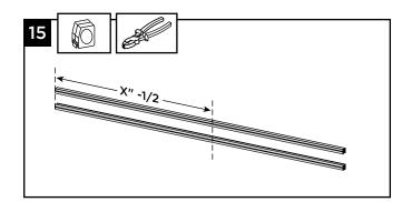
15. Cut both bottom and top rail gaskets to length from previous step.
