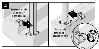
4. Center lower stair bracket on post above the marked line and attach using two self-tapping screws *(provided)*. In some cases it may be difficult to attach the stair bracket on the lower stair post. Recommend using a 90° drill adapter or loosen the post to get access to the lower bracket screw holes.
