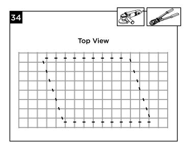
34.Cut mesh at all marks using heavy-duty bolt cutters or angle grinder.
