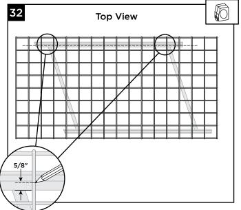
32.At inside of top rail measure **UP** 5/8" and mark mesh at this location. Do this at opposite end of mesh panel/top rail. Using straight edge, mark **MESH ONLY** at all intersection points.
