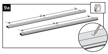
9a.Measure the distance between the vertical end holes on **both top and bottom rails**. Mark the center.
