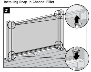
21. Cut snap-in channel filler to correct length and install into channels of bottom and top rails. Use of a rubber mallet may assist with this step. **DO NOT** attempt to cut short snap-in pieces with a miter saw. Use an angle grinder or hack saw only. Attachment of Bracket Covers, Skirts, and Caps
