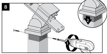
8. Attach stair crossover swivel bracket to post with two self-tapping screws (*provided*). Slide cover over post to hide screws.
