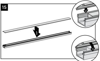
15. Attach "crowned" upper stair rail cover to upper stair rail by aligning cover on one side of rail. Then starting from one end of stair rail, snap cover onto opposing slot working down length of stair rail. GENTLE tapping with a rubber mallet may facilitate fastening.
