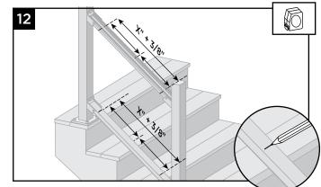
12. Measure and mark the mid-line (6' sections) of the two end marks of the top and bottom rail. Take that measurement and add 3/8" for rod length in next step.
