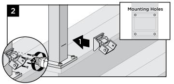
Center lower stair swivel bracket on post above the marked line and attach using four self-tapping screws (*provided*). In some cases it may be difficult to attach the stair bracket on the lower stair post.
