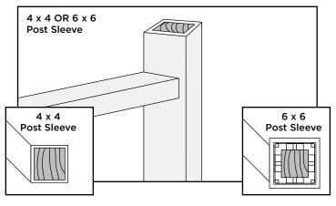
Both 4" x 4" (102 mm x 102 mm) or 6" x 6" (152 mm x 152 mm) post sleeves work well for angles up to 45 degrees. Bottom rail brackets may need to be slightly offset to one side in order to fit properly to hold rail in place. Before attaching bracket to rail, measure and mark to ensure bottom rail remains parallel to upper rail.
