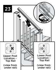
24. Slide baluster spacer up and snap into top rail.
