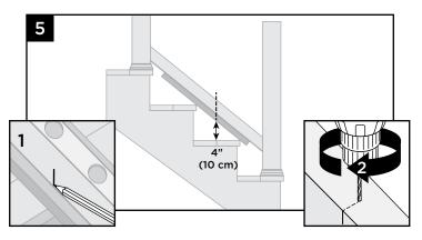
5. Mark approximate location for Foot Block, allowing a measurement of 4" maximum. Invert the bottom rail, and at marked location drill a hole using a 3/16" drill bit in the center of the channel. Foot Block is to be installed at last step.
