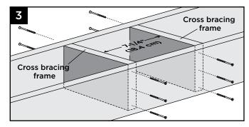
Install two 2" x 8" (51 mm x 203 mm) cross bracing frames in between joists at 7-1/4" (184 mm). Attach a total of twelve 3" (76 mm) pressure-treated compatible screws (not provided).
