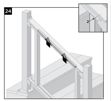
24.Gently tap gasket into channel of top rail. Make sure that vertical is properly aligned with mark on top rail to ensure this is seated in correct location **BEFORE** attaching L-bracket.
