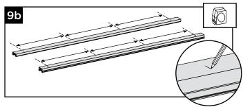
9b.Measure the distance between the vertical end holes on **both top and bottom rails**. Divide the distance into thirds and make two marks on top and bottom rails.
