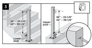
3. On Lower Post - From top of lower bracket, measure up and mark with light line (33-1/4" for 36" rail; 39-1/4" for 42" rail).
