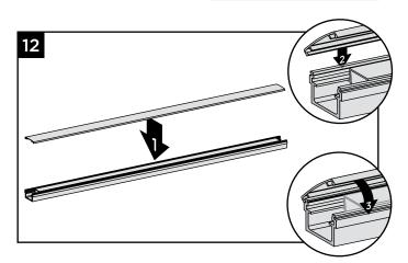
12. Attach "crowned" upper stair rail cover to upper stair rail by aligning cover on one side of rail. Then, starting from one end of stair rail, snap cover onto opposing slot working down length of stair rail. **GENTLY** tapping with a **rubber mallet** may facilitate fastening.
