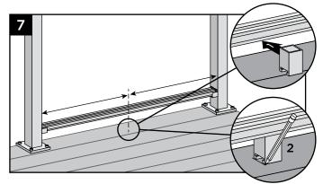
7. Temporarily place bottom rail into lower bracket. To ensure correct location, place Foot Block under center of bottom rail. Mark to provide placement location of base.
