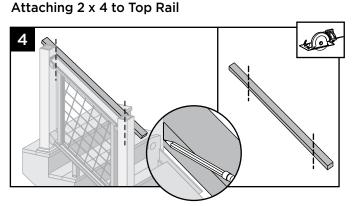
4. Place 2 x 4 beside top rail. Mark and cut (both ends need to be cut on an angle for proper fit).
