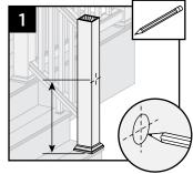
**NOTE:** If deck boards are not installed yet, place a deck board on framing to ensure post sleeve is at correct height.
