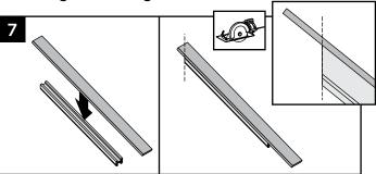
Using the cut top rail as template, cut deck board at upper post location at same angle as the top rail. Leave a generous amount of deck board material at lower post location as this will allow for overhang and can be cut later.
