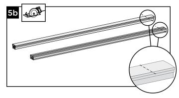
5b. Cut both bottom and top rail to length as determined above.
