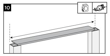
10. Cut deck boards to appropriate length of railing span, remembering to include extra space on each side of the deck board to allow for attachment to the post. Decking boards must cover 1/2 of the pressure-treated post to allow this to be fastened later. If you include extra decking material on each side, this can be cut off later if necessary.
