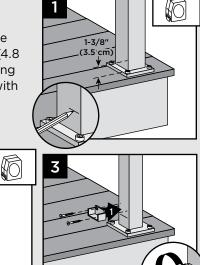
Measure up from post base plate 33-7/16" (84.9 cm) for 36" (92 cm) rail height or 39-7/16" (100.2 cm) for 42" (107 cm) rail height. Mark with light line.
