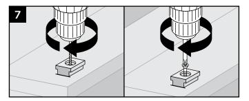
Place base (smaller side facing down) on decking surface. Pre-drill using a 3/16" bit. Attach base of Foot Block using one screw at an angle through base and into decking.  After attached, use a rubber mallet along with scrap piece of wood to tap Foot Block until it locks into place.
