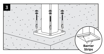
3. Insert the (2) stainless steel barrier strips under the mounting bolt holes. Use appropriate shims if posts are not plumb. Secure post mount with the four expansion anchors, washers and nuts.
