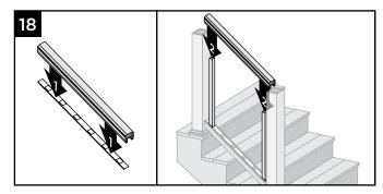
18. Remove baluster spacer from top stair rail and place rail in between posts on top of balusters, ENSURING that balusters remain parallel to post.
