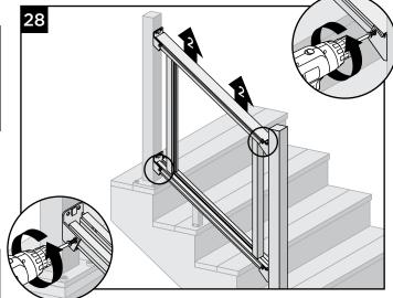
28. Remove the two screws from the brackets that were previously installed in step 9. Remove the railing assembly from the post brackets.
