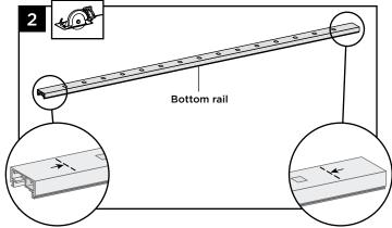
2. Cut bottom rail to the measurement between the bottom swivel brackets.
