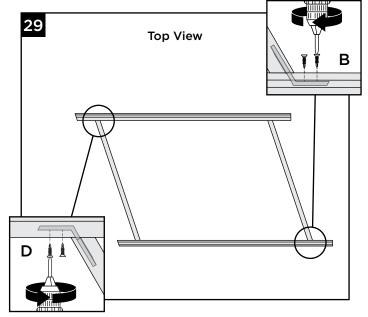
29.Lay railing assembly on large, flat, clean surface. Install remaining L-brackets for section **B** and section **D** into rails where marked using remaining #8 x 5/8" flat head screws (*provided*). Before attachment, verify that verticals align properly with marks.
