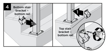
4. Center lower stair bracket on post below the marked line and attach using two #10 x 5/8" self-tapping screws (provided). In some cases it may be difficult to attach the stair bracket on the lower stair post. Recommend using a 90° drill adapter or loosen the post to get access to the lower bracket screw holes.
