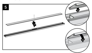
5. Attach "flat" bottom stair rail cover to bottom stair rail. Align cover on one side of the bottom rail in slot on side of rail. Then starting from one end of rail snap cover onto opposing slot working down the length of the rail. In some cases, **GENTLE** tapping with a **rubber mallet** may facilitate fastening.
