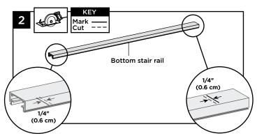
2. Cut each end of the bottom stair rail and bottom rail cover 1/4" (0.6 cm) shorter than the mark on each end to allow for fit into bottom stair rail brackets.
