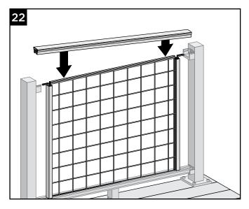
22. Starting at one end and working down, press the top rail firmly onto the top of the mesh panel (with top PVC gasket on mesh). Ensure the top rail is centered properly so top rail will seat into brackets when finished.
