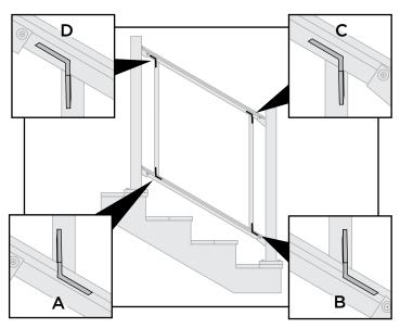
Above is an overall image showing bracket orientation. The next steps will show in detail how to attach them. Refer to corresponding letters in the following steps.
