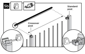
5b. When going from standard-post to crossover post, measurement must be taken from inside of top horizontal swivel bracket to inside lip of crossover bracket (which is attached to top of crossover post).
