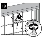
NOTE: Pre-drilling before attachment is recommended.
