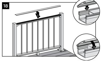
18. Attach "crowned" upper rail cover to upper rail by aligning cover on one side of rail. Then starting from one end of rail, snap cover onto opposing slot working down length of rail. **GENTLE** tapping with a **rubber mallet** may facilitate fastening.
