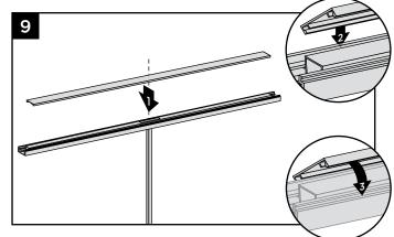
Align cover on one side of bottom rail in slot on side of rail. If using tabbed brackets, the bottom rail cover will also have to be centered on bottom rail to allow for fit into tabbed bracket. Then starting from one end of rail snap cover onto opposing slot working down the length of rail. In some cases, GENTLE tapping with a rubber mallet may facilitate fastening.
