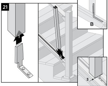
21. **AT BOTTOM POST LOCATION**, place L-bracket into vertical and into channel of bottom rail (L-bracket should be oriented in same direction as previous L-bracket.) Ensure that vertical is seated fully flush with bottom rail, bracket is in the channel, and vertical is aligned with mark on rail.
