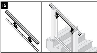
15. Snap baluster spacer into top stair rail. Position top stair rail onto balusters, ensuring balusters are fully seated in rail (position to side of post), and ENSURE that balusters are spaced evenly AND parallel with post. Also allow for a minimum of 1-1/2'' (292 mm) at each end of the stair rail for bracket placement and baluster clearance.
