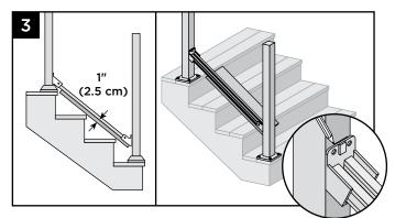
With deck board still on nose of stair tread, place brackets on ends of bottom stair rail (but do not attach) and mark posts for bracket locations.
