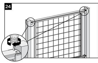
24. Drill two 1/2" holes approximately 1/2" from end of top rail. Repeat this on opposite side of top rail.
