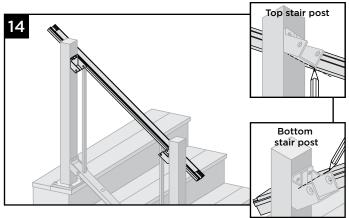
On top stair post location, mark UNDERSIDE of upper rail. On bottom stair post location mark TOPSIDE of upper rail at angled intersection inside the bracket.
