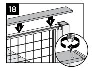
19. Secure boards to top rail using Trex Signature Cocktail Bracket (sold separately). Ensure that there is a bracket at each end of the railing section, then space brackets approximately every 24" and attach with 4 screws provided.
