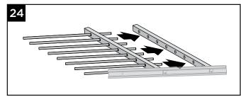
24. Slide rods into lower end and all intermediate verticals.
