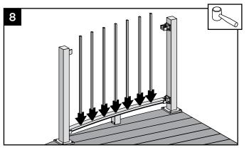
8. Place balusters into holes in lower rail by snapping fully into place.
