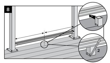
Temporarily place bottom rail into lower bracket. To ensure correct location, place Foot Block under center of bottom rail. Mark to provide placement location of base.
