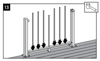
Place remaining balusters into holes in lower rail by snapping fully into place. In some cases, GENTLE tapping with a rubber mallet may facilitate fastening. Attach Upper Railings
