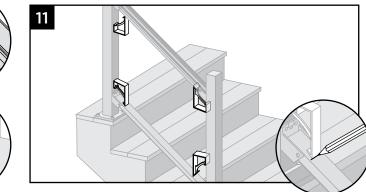
Using the long edge of the stair template, mark the location of the end verticals on the upper and lower rails.
