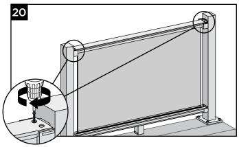
20. Install two #8 x 1-1/4" screws provided into top rail and top bracket on each end of top rail.
