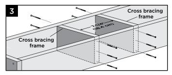
3. Install two 2" x 8" (5.1 cm x 20.3 cm) cross bracing frames in between joists at 7-1/4" (18.4 cm). Attach a total of twelve 3" (7.6 cm) pressure-treated compatible screws (*not provided*).
