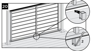
20.Temporarily drop rod rail panel into brackets. To ensure correct location, place Foot Block under center of bottom panel. Mark to provide placement location of base. Once marked remove panel.
