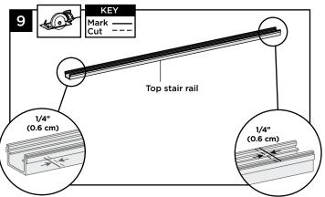
Cut each end of top stair rail and top rail cover 1/4" (0.6 cm) shorter than mark to allow for fit into top stair rail bracket.
