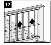
**NOTE:** If necessary, cut tips off rail gaskets prior to installation.
