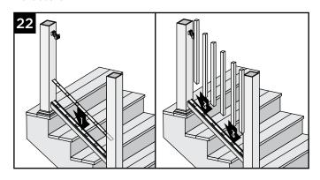
22. Place inverted top baluster spacer on bottom rail rail/baluster spacer, ensuring that baluster holes line up. Install balusters into bottom stair rail.
