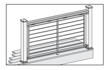
**Important:** ONLY use with Pressure-Treated post, Trex Post Mounts or Trex Joist Mount Post WITH Trex post sleeves. Trex Signature Posts and Joist Mount Posts cannot be used with Rod Rail Traditional.
