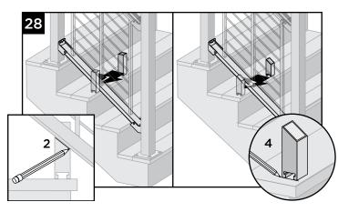
28. Temporarily drop assembled stair rod rail panel into brackets. To ensure proper location place Foot Block towards the nose of the stair tread along the side of the bottom rail. Mark location of angle on Foot Block and cut on mark. Then place Foot Block under the center of the bottom rail. Mark placement location of the base.
