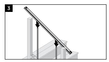
3. Position top stair rail onto balusters ensuring balusters are fully seated in top rail (position to side of post) and **ENSURE** that balusters are parallel with post.
