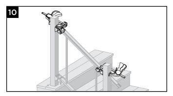
10. Clamp brackets to side of rail with brackets in correct swivel location/angle (this is important to ensure correct location of swivel brackets).
