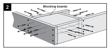
Install two 2" x 8" (5.1 cm x 20.3 cm) boards as blocking under post location. Securely attach blocking using a total of twenty-four 3" (7.6 cm) pressure-treated compatible screws (not provided).
