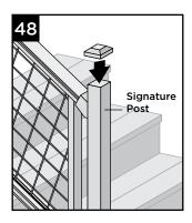
49.Attach post caps to post sleeves using external- grade PVC construction adhesive (apply adhesive on the inside self-centering/ corner tabs).
