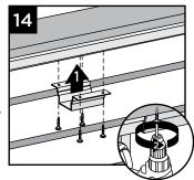
NOTE: Pre-drilling before attachment is recommended.
