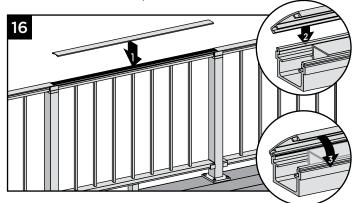
16. Attach "crowned" upper rail cover to upper rail by aligning cover on one side of rail. Then starting from one end of rail, snap cover onto opposing slot working down length of rail. GENTLE tapping with a rubber mallet may facilitate fastening.
