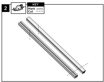
2. Cut both bottom and top rails to same length. ENSURE POSTS ARE PLUMB before cutting.
