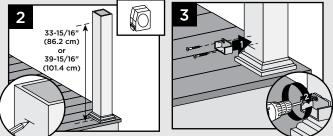
Measure up from decking surface 33-15/16" (862 cm) for 36" (92 cm) rail height or 39-15/16" (101.4 cm) for 42" (107 cm) rail height. Mark with light line.
