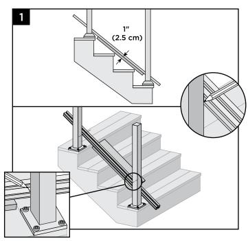
Place a 1" deck board along the nose of the stair tread, then lay the bottom stair rail on top of the deck board. Use the lower and upper stair post to determine the length of the bottom stair rail. At LOWER STAIR POST, mark on topside of rail and cut PERPENDICULAR to the rail. At UPPER STAIR POST, mark on INTERSECTION/SIDE OF RAIL AND CUT RAIL TO THIS ANGLE.
