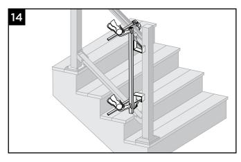
14. Clamp first vertical (lower part of stairs) in place, using width of stair template to position.
