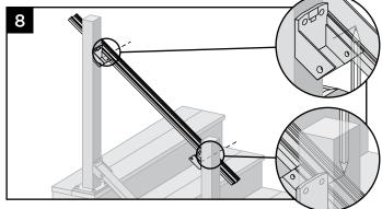
8. Position top rail to side of post. Mark top stair rail at each location stated. On **UPPER STAIR POST**, mark from underside of bottom rail. On **LOWER STAIR POST**, mark from topside of bottom rail.
