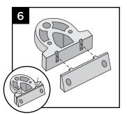
**TIP:** Use a dap of super glue when snapping bracket together. This will help stabilize bracket when installing.
