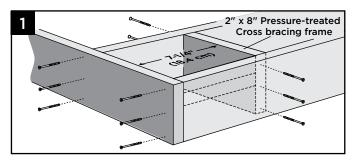
Install 2" x 8" (5.1 cm x 20.3 cm) cross bracing frame in between joists at 7-1/4" (18.4 cm). Attach a total of twelve 3" (7.6 cm) pressure-treated compatible screws (not provided).
