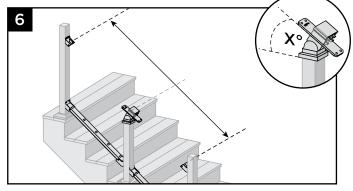
6. Determine location/height of the stair crossover swivel bracket by aligning the angle of this with the fixed brackets (or compound swivel brackets) already installed (posts can be cut if necessary).
