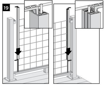
19. Slide vertical supports down onto vertical PVC gaskets, also ensuring that L-bracket is fully seated into bottom rail channel. Light tapping with rubber mallet may be required.
