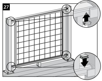
27. Cut snap-in channel filler to correct length at each location and install into channels of bottom and top rails. Use of a rubber mallet may assist with this step. **DO NOT** attempt to cut short snap in pieces with a miter saw. Use an angle grinder or hack saw only.
