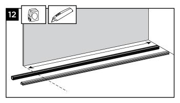
12. Cut both bottom sill gasket and top head gasket to the same length of glass panel.
