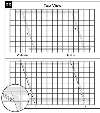
33. For the vertical measurements, align straight edge with **OUTSIDE** of one vertical and mark mesh at all intersection points. Align straight edge with **INSIDE** of opposite vertical and mark mesh at all intersection points.
