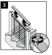
THE UNDERSIDE OR SLIGHT PLANING ON THE UNDERSIDE TO ALLOW DECK BOARD TO CLEAR TOPS OF BRACKETS AND SIT FLUSH ON TOP OF POSTS AND RAILS. Attach boards on each post with Trex-recommended composite screws (quantity of 2 per each post/board end).
