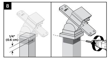
8. Once location/height is determined, center and predrill two holes (using a drill bit slightly smaller than that of self-tapping screw diameter) on opposite sides of post, approximately. 1/4" (0.6 cm) from top of post. Drill through the post and into the stair crossover swivel bracket on each side.
