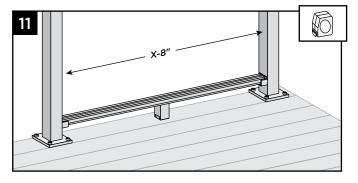
11. If not installing full span, mesh will require cutting from equal distance on each side. Measure distance between posts and subtract 8".
