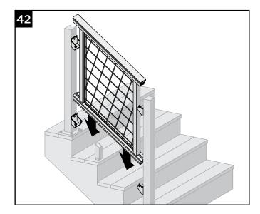
42. Drop assembled stair mesh rail panel into brackets. Ensure that rails are fully seated into brackets and verticals are completely seated on rails.
