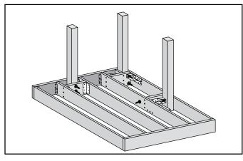
**NOTE:** To allow fascia to sit flat against framing, route/trim out back side of fascia to allow for fit over bolt locations.
