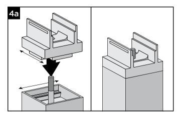
4a. Place the line crossover bracket over the bolt onto the end of the post.
