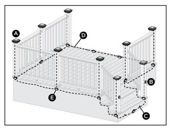
**NOTE:** All wiring and splitters are mounted to the inside of framing. Picture above is a general representation of where to place them.
