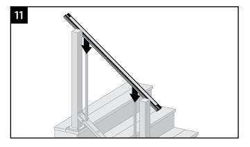
Position top stair rail onto balusters ensuring balusters are fully seated in top rail (position to side of post) and ENSURE that balusters are parallel with post.
