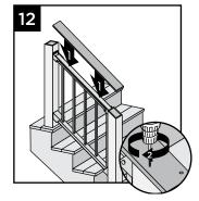
PLANING ON THE UNDERSIDE TO ALLOW DECK BOARD TO CLEAR TOPS OF BRACKETS AND SIT FLUSH ON TOP OF POSTS AND RAILS. Attach boards on each post with Trex-recommended composite screws (quantity of 2 per each board end).
