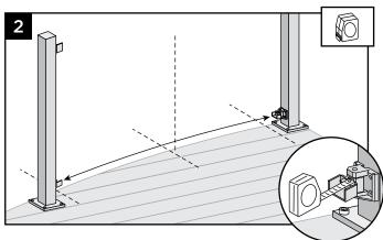
With brackets in correct swivel location, measure distance from inside of bracket to inside of bracket.
