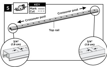
5. Cut each end of top rail 3/4" (1.9 cm) **LONGER** than the mark to allow for fit into the crossover post bracket on each side.
