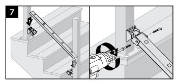
7. Set bottom stair rail into bottom stair rail brackets. Attach bottom stair rail to bottom stair bracket using two self-tapping screws (*provided*) on each side of bracket.
