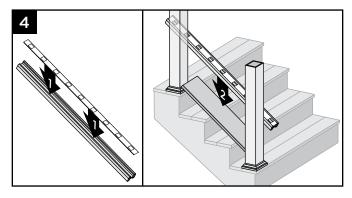
4. Snap baluster spacer into bottom stair rail and lay bottom stair rail on top of the deck board.
