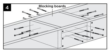
Install two 2" x 8" (5.1 cm x 20.3 cm) boards as blocking under post location. Securely attach blocking using a total of twenty-four 3" (7.6 cm) pressure-treated compatible screws (not provided).
