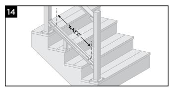
14. Measure distance between marked lines on bottom rail and subtract 1/2" from this measurement.
