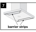
Attach posts using four 3/8" x 6" (1 cm x 15.2 cm) hex cap bolts, washers, and nuts, along with aluminum back plate on underside of blocking. If the project requires IRC compliance, this back plate MUST be installed under the decking to ensure this will meet code compliance. Reference SKU part number ALPOSTHWDECK for required hardware and
