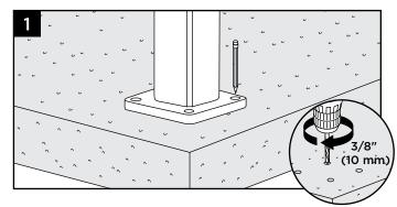
Using post as a template, mark locations of the four holes and drill into concrete at least 2-5/8" (66.7 mm) using a 3/8" (10 mm) masonry bit.
