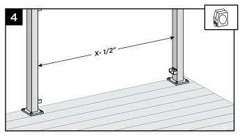
4. Measure distance between posts (X), and subtract 1/2'' for bracket clearance.
