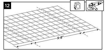
12. Cut mesh panel to this measurement, again cutting equal distances from each side so mesh is centered.
