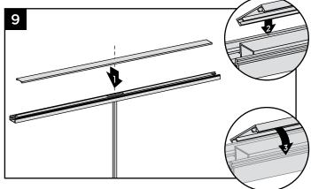
9. Align cover on one side of bottom rail in slot on side of rail. If using tabbed brackets, the bottom rail cover will also have to be centered on bottom rail to allow for fit into tabbed bracket. Then starting from one end of rail snap cover onto opposing slot working down the length of rail. In some cases, **GENTLE** tapping with a **rubber mallet** may facilitate fastening.
