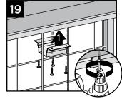
NOTE: Pre-drilling before attachment is recommended.
