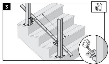
3. With brackets in correct swivel locations, measure distance from inside of swivel bracket to inside of swivel bracket. Ensure that before cutting, balusters holes are parallel and centered in between the posts and also allow for clearance for attachment to brackets. Mark bottom stair rail at each intersection.
