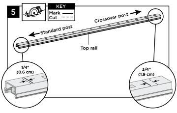
Top rail must be cut differently on each side of the rail. Railing side that attaches to standard post should be cut 1/4" (0.6 cm) shorter than the mark to allow for fit into top rail bracket. Railing side that attaches to the crossover post should be cut 3/4" (1.9 cm) LONGER than the mark to allow for fit into the crossover post bracket.
