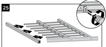
25. Slide upper end vertical onto rods and attach to bottom rail using ST Wedge Spacer and screws provided.
