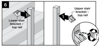
6. Center upper stair brackets on posts **below** the marked lines and attach using two self-tapping screws (*provided*).
