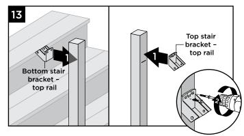
Remove upper stair rail and center upper stair fixed bracket on post **above** the marked line and attach using two self-tapping screws (*provided*).
