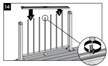
14. Working from one end of upper rail, snap balusters into upper rail working down length of rail. Fasten center baluster into center slot using two  $#8 \times 1-1/4''$ (3.2 cm) screws (provided).
