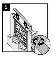
NOTCH CUT ON THE UNDERSIDE OR SLIGHT PLANING ON THE UNDERSIDE TO ALLOW DECK BOARD TO CLEAR TOPS OF BRACKETS AND SIT FLUSH ON TOP OF POSTS AND RAILS. Attach boards on each post with Trex-recommended composite screws (quantity of 2 per each post/ board end).
