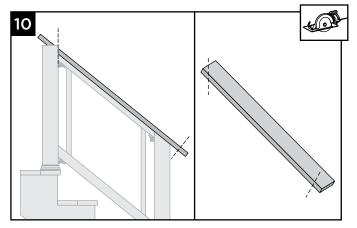
10.Measure accordingly and cut deck boards to appropriate length of railing span also allowing for additional decking material that will be installed over the lower stair rail post.
