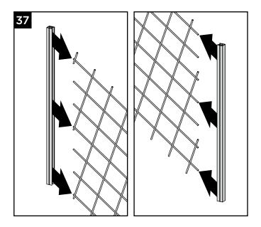
37.Attach vertical gaskets to each side of mesh panel. Make sure gaskets are fully seated onto mesh.
