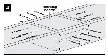
Install two 2" x 8" (51 mm x 203 mm) boards as blocking under post location. Securely attach blocking using a total of twenty-four 3" (76 mm) pressure- treated compatible screws (not provided).
