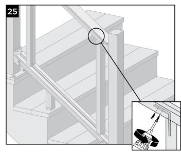
25.Attach L-bracket to top rail using two #8 x 5/8" flat head screws (*provided*).
