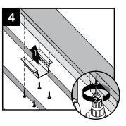
NOTE: Pre-drilling before attachment is recommended.
