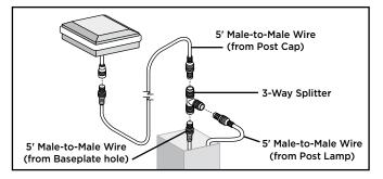
**NOTE:** If connecting a Trex Wedge Deck Rail Light as well, a 3-way adapter and extra 5' male-to-male wire (not provided) can be used inside the post so that only one wire must be run through the hole in the base of the post (and post blocking). This is optional.
