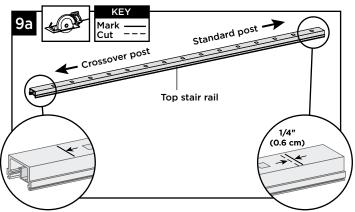
9a. Top stair rail along with rail insert must be cut differently on each side of the rail. Railing side that attaches to standard post should be cut 1/4" (0.6 cm) shorter than the mark to allow for fit into top rail bracket. Railing side that attaches to the crossover post should be cut directly on the mark to allow for fit into the crossover post bracket.
