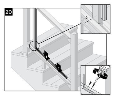
20. Gently tap gasket into channel of bottom rail. Make sure that upper vertical is properly aligned with mark on bottom rail to ensure this is seated in correct location **BEFORE** attaching L-bracket. Attach L-bracket to bottom rail with two #8 x 5/8" flat head screws (*provided*).
