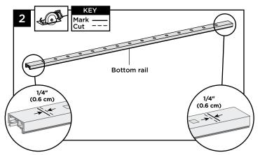
2. Cut each end of bottom rail 1/4" (0.6 cm) shorter than mark on each end to allow for fit into bottom rail brackets.
