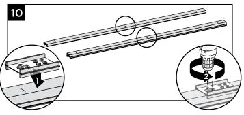
10. Using the slot on the HZ template, locate marked line and drill two 7/64" pilot holes (or mark with a punch).
