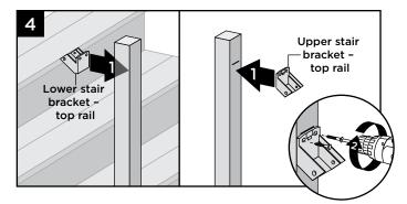
4. Center upper stair brackets on posts **below** the marked lines and attach using two self-tapping screws (*provided*).
