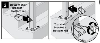
Center lower stair bracket on post above the marked line and attach using two self-tapping screws (provided). In some cases it may be difficult to attach the stair bracket on the lower stair post. A 90° cordless drill is recommended to attach screws in this area.
