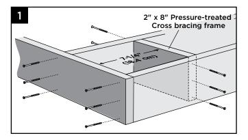
Install 2" x 8" (51 mm x 203 mm) cross bracing frame in between joists at 7-1/4" (184 mm). Attach a total of twelve 3" (76 mm) pressure-treated compatible screws (not provided).
