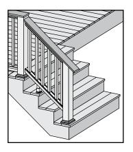
» DO NOT CUT POST/POST SLEEVES UNTIL TOP RAIL IS FULLY INSTALLED. THE DECK BOARD USED IN TRANSCEND STAIR COCKTAIL RAILING WILL NEED TO TERMINATE AT THE TOP OF THE POST AS SHOWN ABOVE. THE DECK BOARD WILL HAVE TO BE INSTALLED INTO THE SIDE OF THE POST IN THESE AREAS USING 2 APPROPRIATE COMPOSITE DECKING SCREWS - PRE-DRILLING IS RECOMMENDED.
