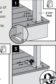
Measure up from post base plate 33-7/16" (84.9 cm) for 36" (92 cm) rail height or 39-7/16" (100.2 cm) for 42" (107 cm) rail height. Mark with light line.
