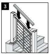
Secure 2 x 4 to top rail using Trex Signature<sup>™</sup> Cocktail Bracket (sold separately). Ensure that there is a bracket at each end of the railing section, then space brackets approximately every 24" and attach with 4 screws provided.
