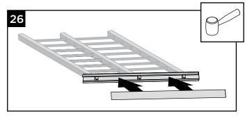
26. Using a mallet, install bottom rail cover onto bottom rail.
