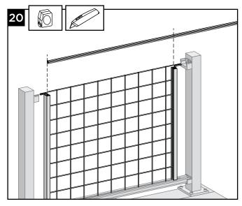
20. Using razor knife, cut top PVC gasket the same length as mesh panel.
