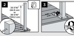
Measure up from post base plate 33-7/16" (84.9 cm) for 36" (92 cm) rail height or 39-7/16" (100.2 cm) for 42" (107 cm) rail height. Mark with light line.
