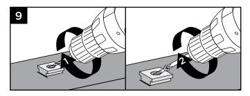
9. Remove bottom rail from lower brackets. Place base (smaller side facing down) on decking surface. Predrill using a 3/16" bit. Attach base of Foot Block using one screw at an angle through base and into decking.
