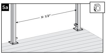
5a. Measure distance between posts (X), and subtract 1/2'' for bracket clearance.
