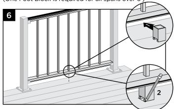
6. Temporarily place panel onto brackets. To ensure correct location, place Foot Block under center of bottom panel rail. Mark to provide placement location of base.
