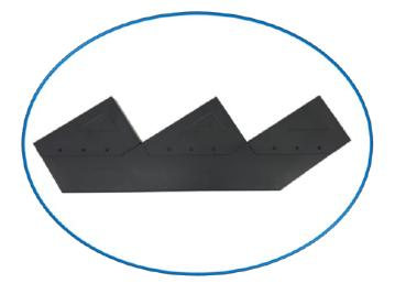
Use a metal cutting saw and blade to make the marked cuts.
